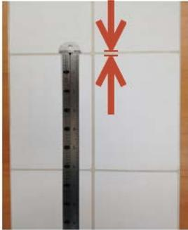
Measure this distance and input into **Gutter**
