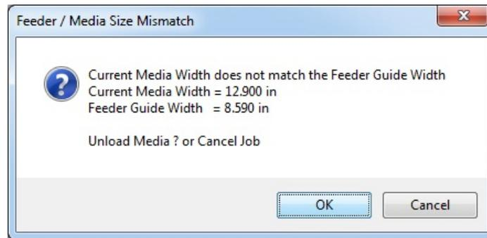
If a previous media width was used with your feeder, the Feeder Guide will retain that width. If the new media width is not the same size then the Feeder / Media Size Mismatch window will display. Select **OK** to Unload Media (If there is no media loaded this action still needs to be completed).
