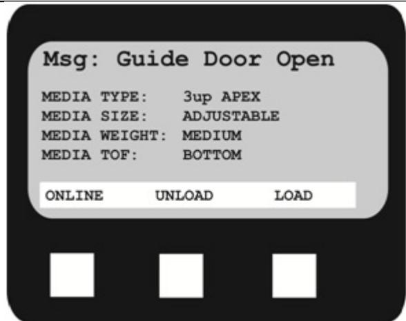
The control panel screen should look like this after the load finishes:
